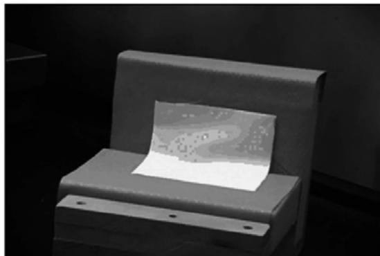
**Section 2** covering the Barrier Materials Test measures the tendency of the barrier material to smolder after exposure to smoldering cigarettes under specified conditions. Type 2 cover fabric is wrapped around the candidate barrier material
